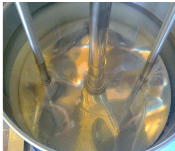
Fig. 4. Molten vaseline on installation “Thermobat -M”.
