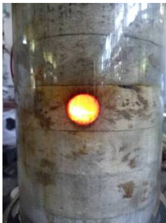
Fig.1. The laboratory reactor for thermal purification.
