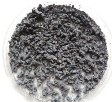
Fig. 1. Photo of \text{CoFe}_2\text{O}_4 particles after annealing
