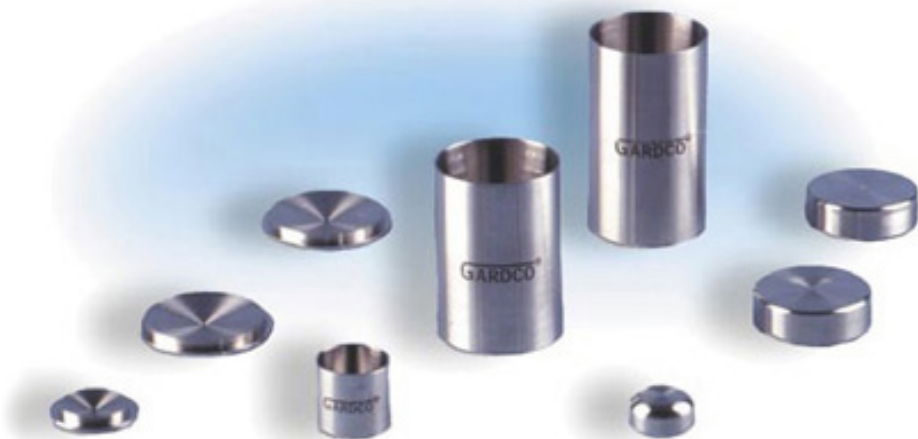
1.23 pav. Standartizuotos MR matavimo talpos (weight per gallon cup) [57]
