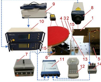
Figure 6. A schematic diagram of the experimental setup used for ME-PEH characterization: 1 – transducer (Piezo Systems T226-A4-503Y), 2 – magnetic tip mass (driven magnet), 3 – driving magnet; 4 – rotating table, 5 – micro-positioning stage, 6 – DC motor, 7 – DC power supply (Mastech HY3020E), 8 – LDV sensor head (Polytec OFV-505), 9 – Rotational LDV sensor head (Polytec RLV-500), 10 – LDV controllers (Polytec OFV-5000 and RLV-5000), 11 – 4-channel digital oscilloscope (PICO 6403); 12 – Magnetometer (Magnet-Physik FH-54); 13 – magnetometer sensor (transverse Hall probe HS-TGB5); 14 – adjustable resistance box (IET LABS RS-200-SC); 15 – retroreflective tape.
