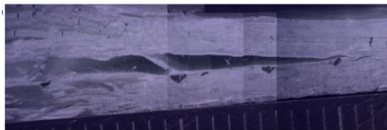
Figure 2-6. Composite material ageing effects [40]
