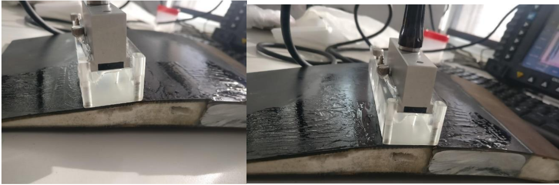
Figure 5-28. Artificial polyurethane foam defects and phased array setup during inspection
