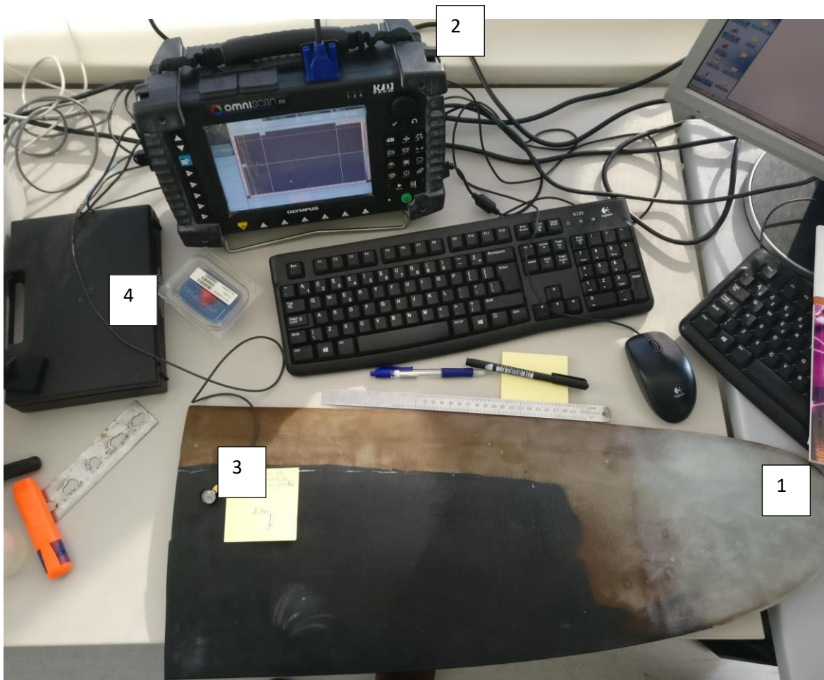
Figure 4-2. Propeller inspection set-up
