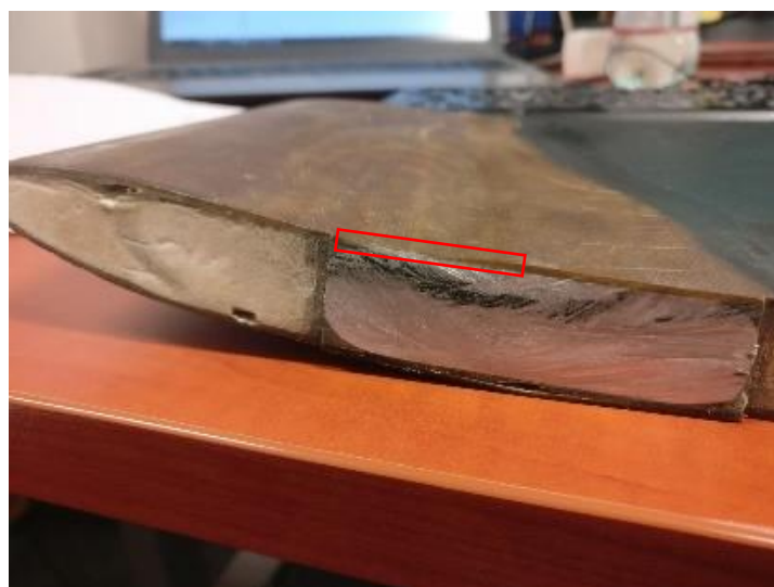
Figure 5-32 – Fiberglass shell blend-out performed to inspect the phased array resolution and sensitivity
