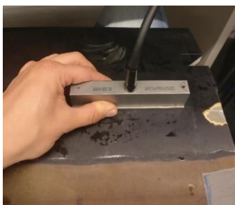
Figure 5-2. Location of the PA during inspection
