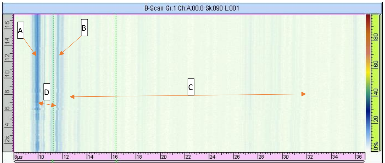
Figure 5-9. 5 MHz PA inspection for fiberglass-foam-fiberglass layers
