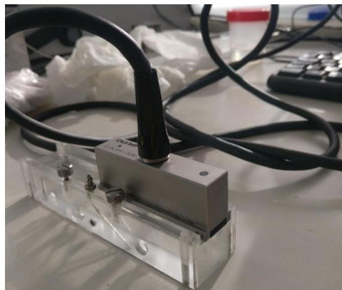
Figure 5-19. 3.5 MHz and wedge setup
