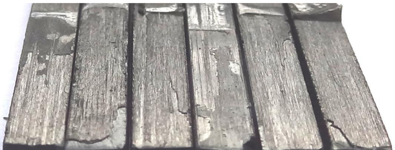
Fig. 41. Views of adhesion zones after fatigue fracture [1]
