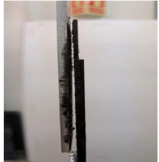
Fig. 24. Adhesive failure with AA2024-T3(left) and mixed CFR bonded connections(right) [31]
