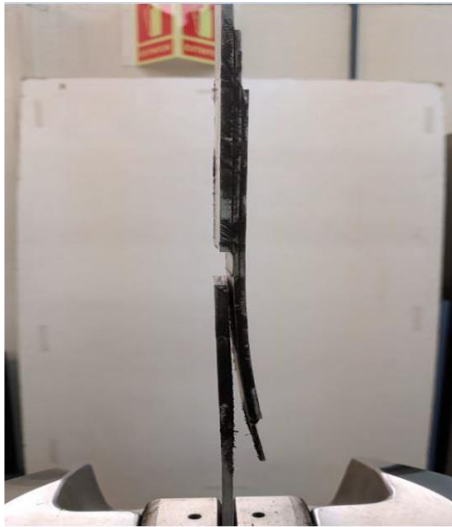
Fig. 24. Adhesive failure with AA2024-T3(left) and mixed CFR bonded connections(right) [31]
