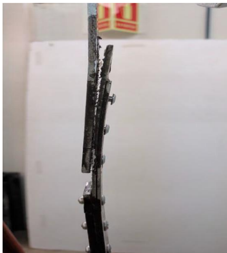
Fig. 25. Hybrid joint failure with AA2024-T3(left) and mixed CFRE(right) [31]
