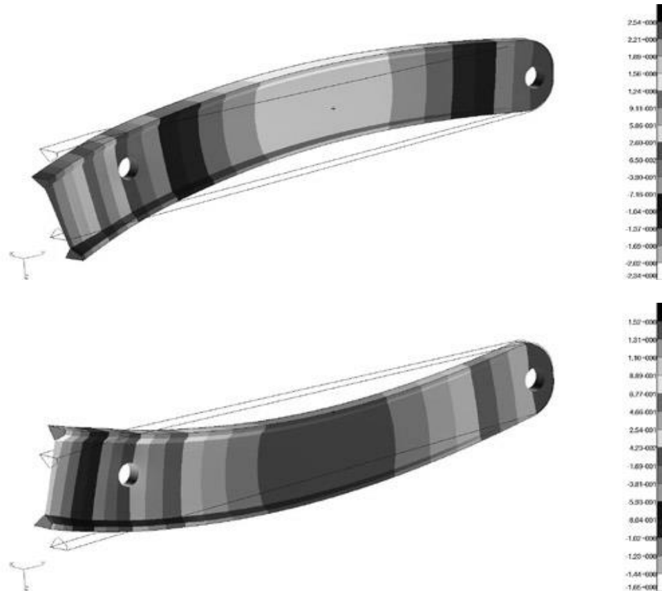
Fig. 12. Result of FEM analysis. Load factor n = 5.7 and -3.7 [27]
