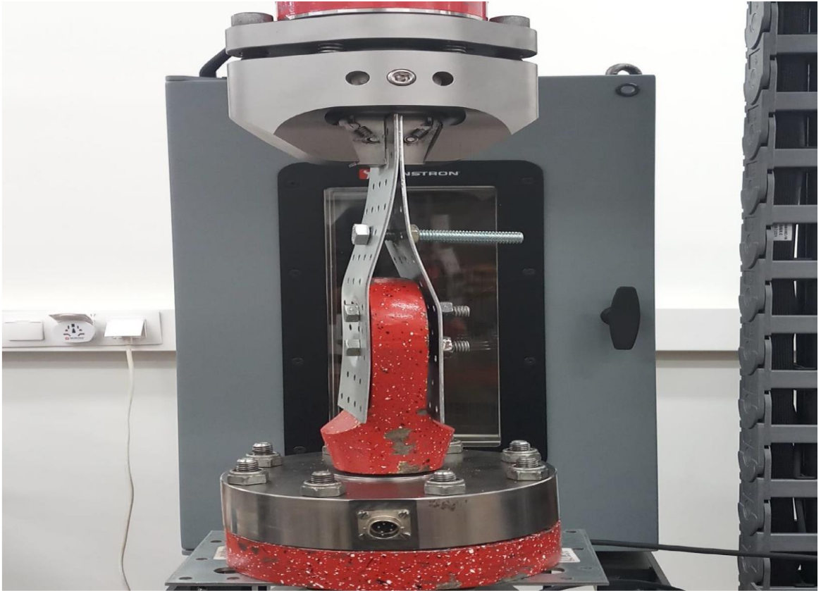
Figure. Calibration of the load cell (MK11-50KN)
