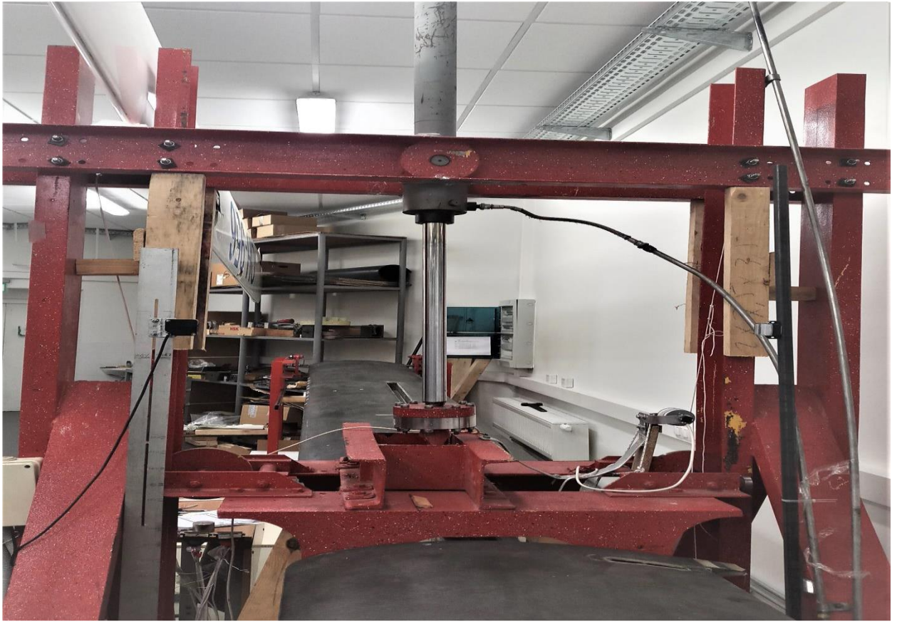
Figure. Experimental setup of a sailplane wing
