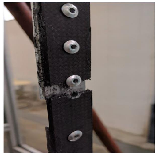
Fig. 25. Hybrid joint failure with AA2024-T3(left) and mixed CFRE(right) [31]
