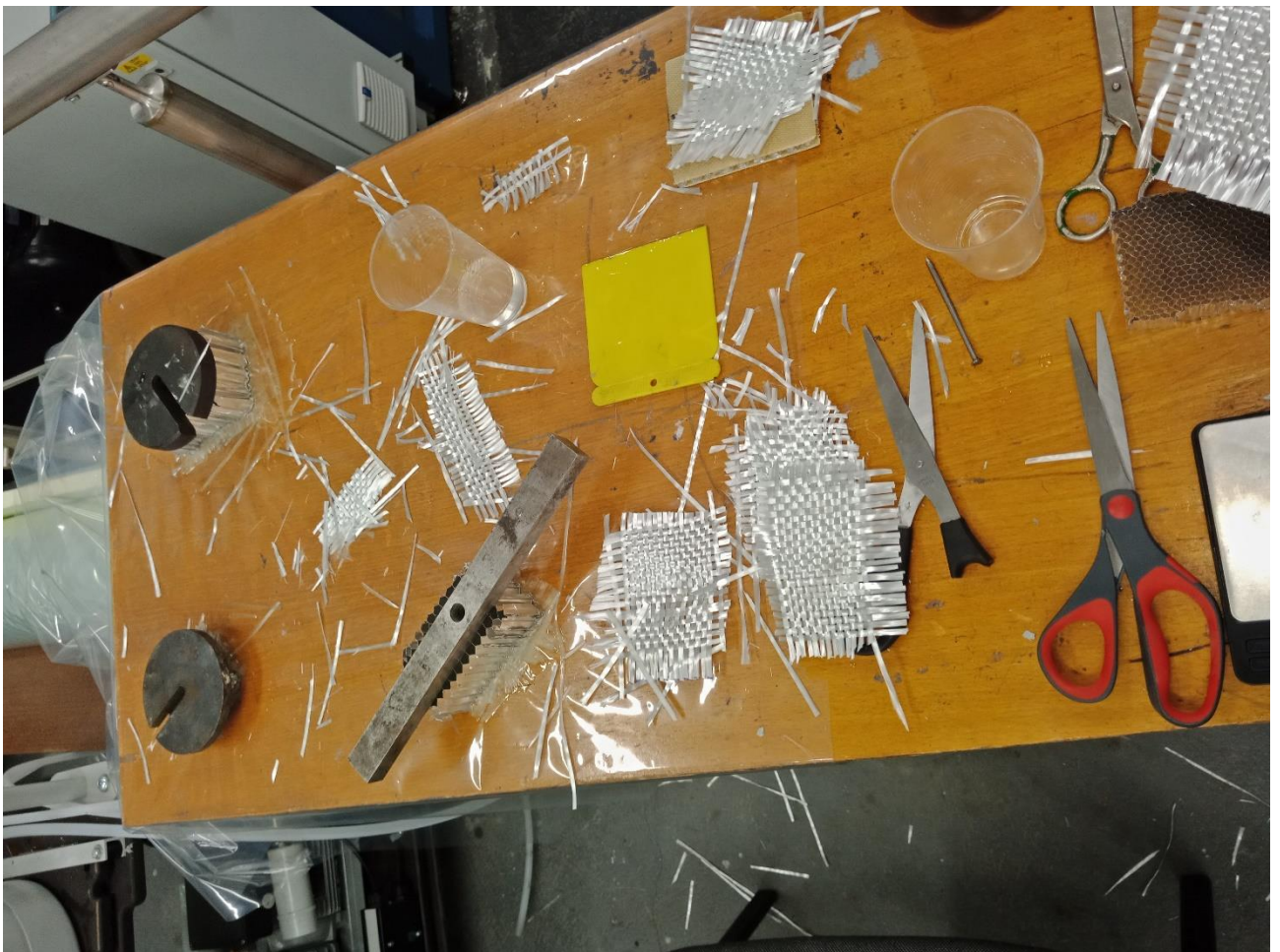
Fig.3. 14. Fabrication of Honeycomb with glass fibre.
