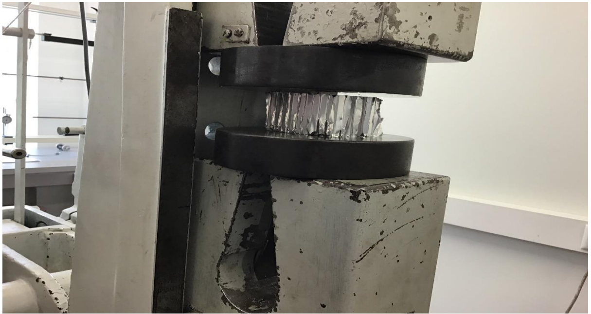
Fig.3. 7. Honeycomb Structure clamped for compression test.
