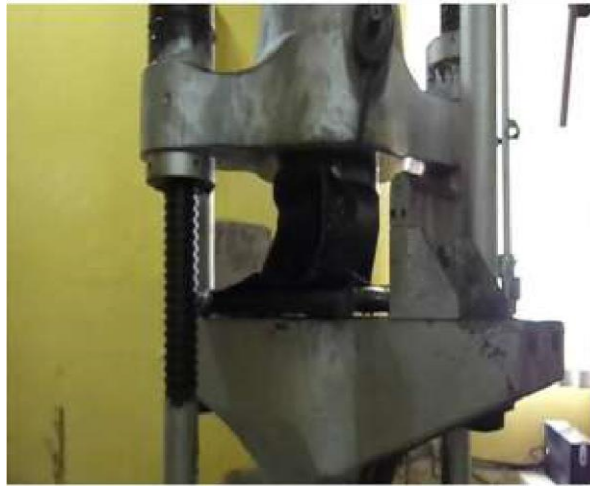
Fig.1. 9. Midway Crushing of Impact Attenuator on UTM.
