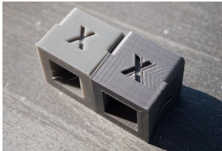
Fig 15. Part with no surface ringing on the left and part with ringing on the right [16]
