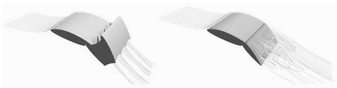
Fig. 14. Airflow comparison of integrated and conventional high lift device (18)
