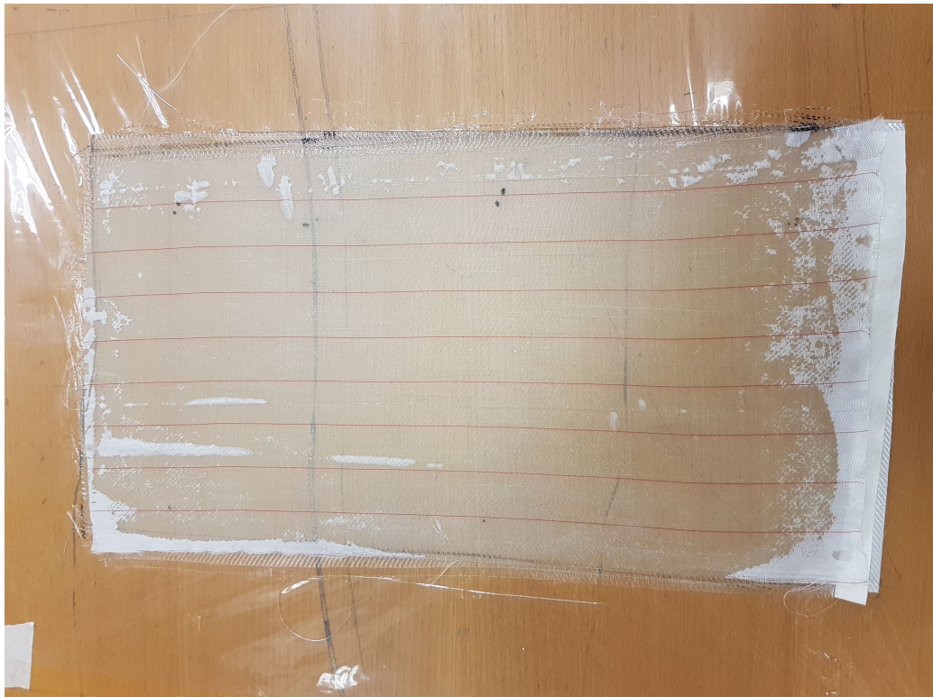
Fig. 2.9 Non-stick fabric used for panel production
