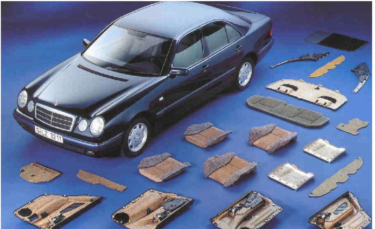
Fig. 1.9 Parts manufactured utilizing bio-composites in Mercedes-Benz vehicle [22]
