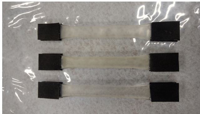
Fig. 2.1 PMMA resin tensile test specimens.
