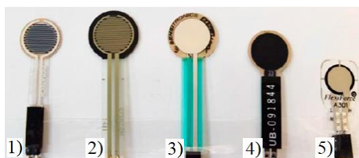
1.10 pav. Slėgio jutikliai: 1 – Peratech QTC™; 2 – Interlink FSR®; 3 – Sensitronics® FSR; 4 – Tactilus® Sensor; 5 – Tekscan Flex [42]
