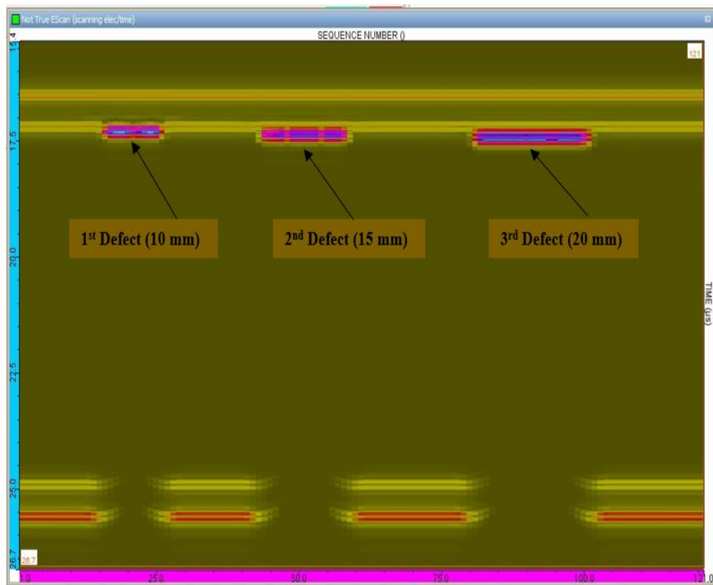
Fig 29. Scan view of defects on model.
