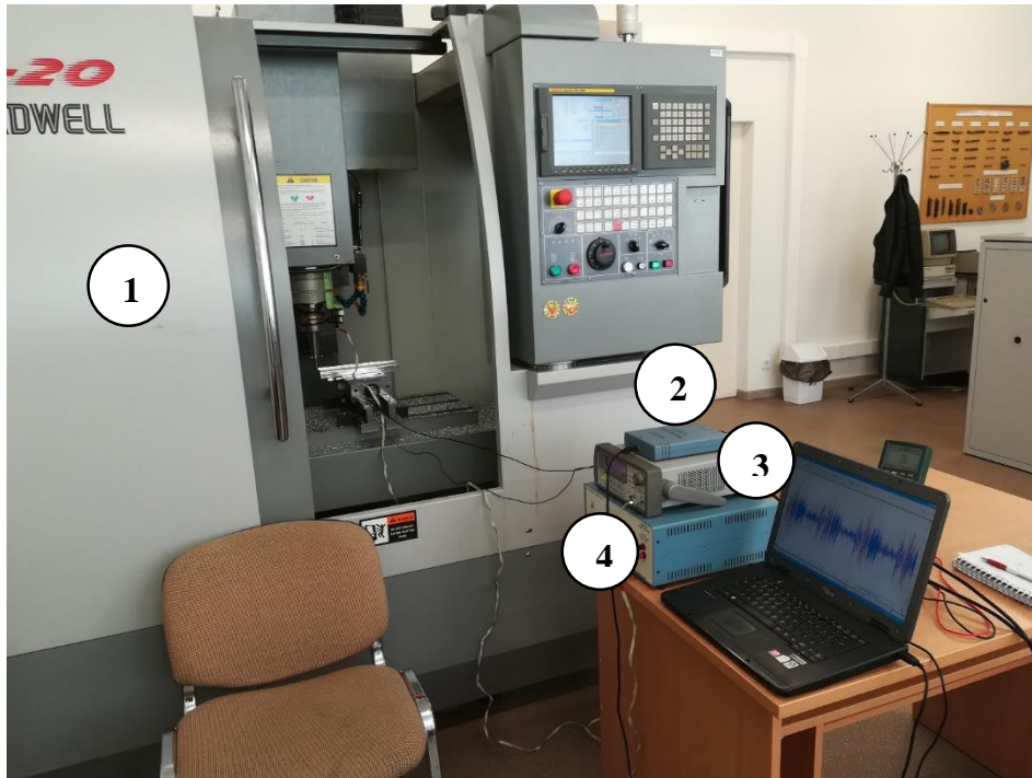
Figure 27. Experiment setup (I): 1 – Leadwell V-20 CNC machining center [37], 2 – Picoscope oscilloscope, 3 – Arbitrary waveform generator Agilent 33220A, 20MHz [38], 4 –Linear amplifier Piezo Systems model EPA-104 [39].
