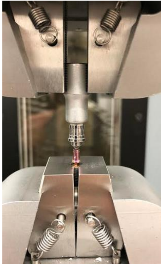
Fig. 22. Implant in the machine holder
