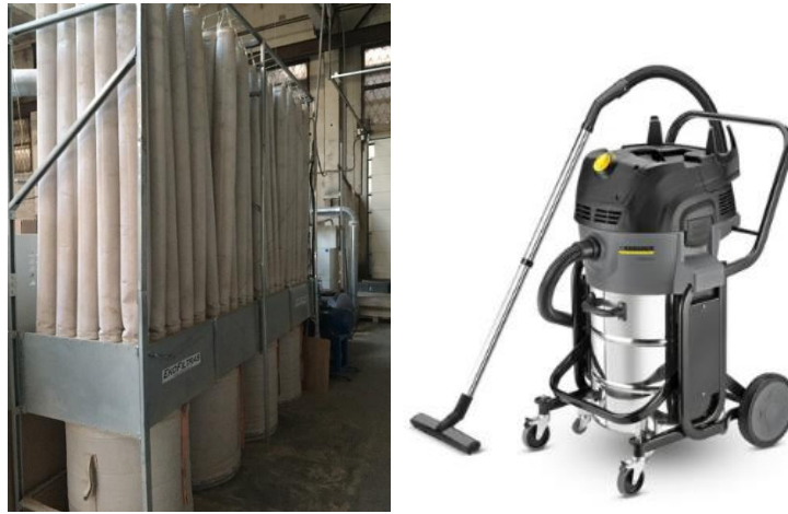
Fig. 27 On the left: Dust removal machine; On the right: Special wood dust vacuum [33]
