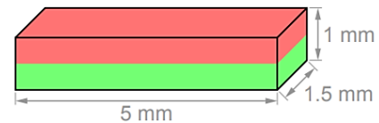
Fig.34. Chosen magnet for contactless excitation [54]
