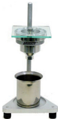
Fig. 12. The Ford cup apparatus late 2000 model (43)
