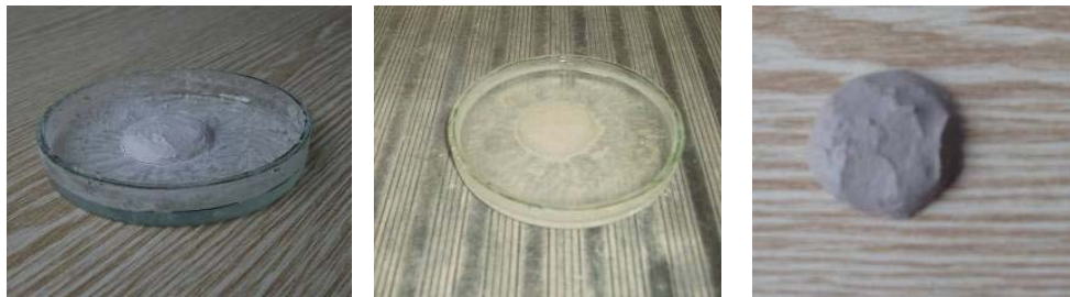
Figure 1. View of filler aggregate samples during the activity detection: filler aggregate and paste of hydrated lime putty in an air (left); filler aggregate and paste of hydrated lime putty in water (centre); filler aggregate and paste of hydrated lime putty after investigations (right)
