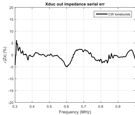
Fig. 20. Transducer output impedance measurement errors when rectangular CW tonebursts are used, R_L 330 \Omega , R_H 100k \Omega case.
