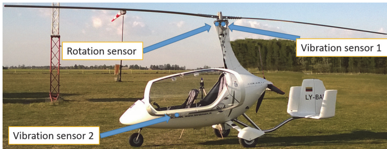
Fig. 2. Vibrations and rotation sensors location on autogyro Calidus [5]
