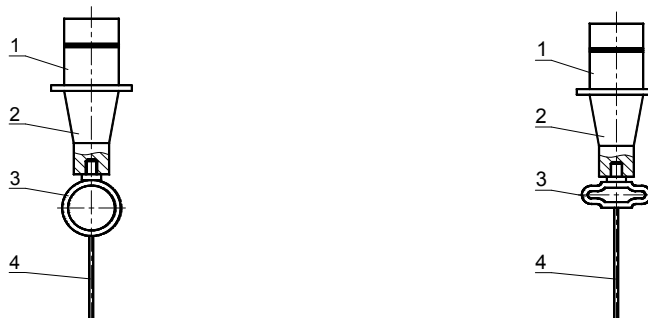
Fig. 1. Schematics of acoustic tools with elastic concentrators: 1 – piezoceramic transducer, 2 – conical concentrator, 3 – intermediate elastic loop shaped concentrator in the form of a circular ring or a loop with parallel sides; 4 – rod shaped tip of the instrument
