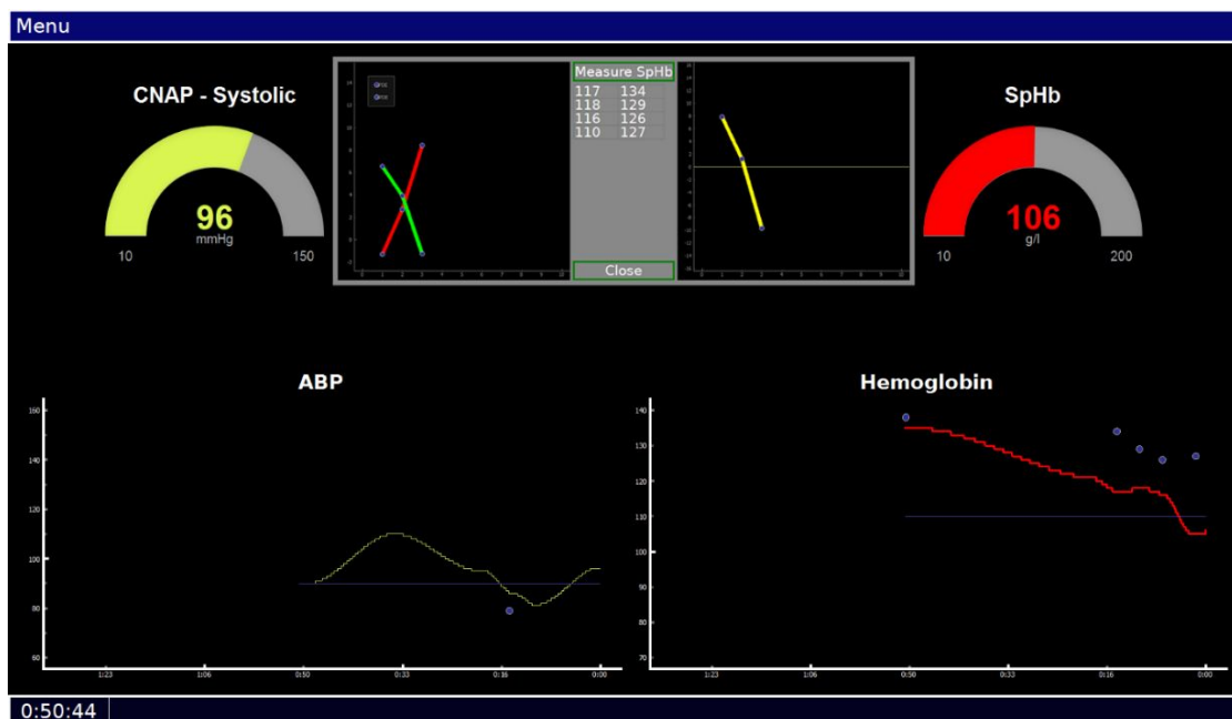
Fig. 2. User interface. The screen continuously displays the real time non-invasive readings of systolic ABP and SpHb, as well as their trends over time. The pop-up window shows plasma dilution efficacy trends during the mVLT protocol.
