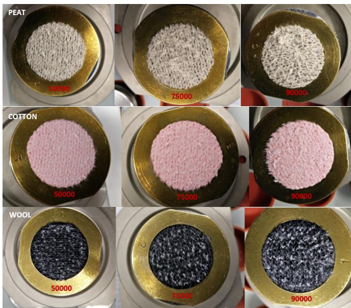
Figure 10. Surface view of pure peat, cotton and woollen knits after 5 \times 10^4 , 7.5 \times 10^4 , and 9 \times 10^4 revolutions during the abrasion resistance test
