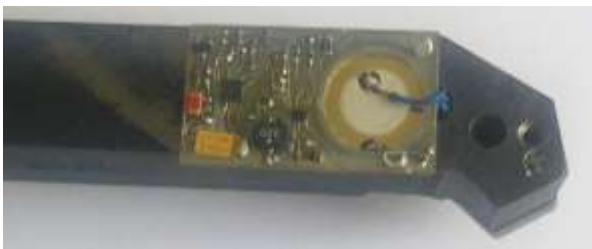
Fig. 13 Self-powered wireless sensor node on turning tool
