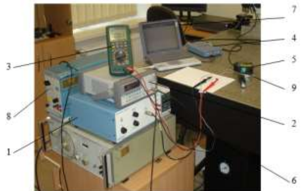
Fig. 4 Experimental equipment: 1 - signal amplifier EPA-104; 2 - signal generator Agilent 33220A; 3 - multimeter Mastech MS8218; 4 - oscilloscope "PicoScope-3424"; 5 - laser displacement sensor LK-G82; 6 - controller LK-G3001PV; 7 - PC; 8 - power source; 9 - piezoelectric acoustic generator KBS - 15 DB - 4 A
