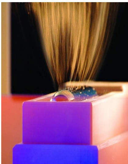
Figure 1. Electrospinning process of “Nanospider™” equipment [17].
