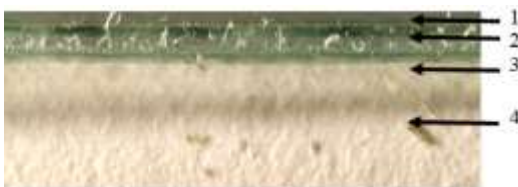
Fig. 2 Cross section image of the MRP data page of a travel document used by some EU countries. 1 - protective polycarbonate transparent layer, thickness of which varies in the range of 50 – 100 \mu\text{m} ; 2 - polycarbonate transparent layer for data recording of the thickness 100 – 150 \mu\text{m} ; 3 - polycarbonate white layer of the thickness 200 – 550 \mu\text{m} ; 4 - protective teslin layer of the thickness 400 – 450 \mu\text{m} . [11]
