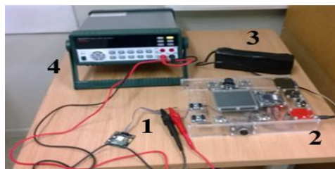
Fig. 3. Implementation view 1 -CM, 2 – CPM, 3 – PS, 4 – multimeter.
