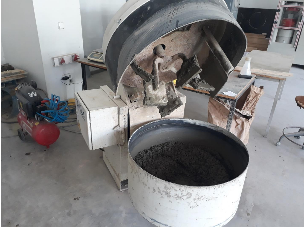
Figure 11: Concrete mixing in “Zyclos” mixer
