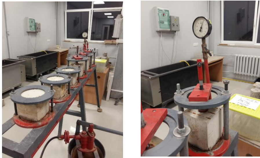
Figure 12: Water impermeability test in special frame
