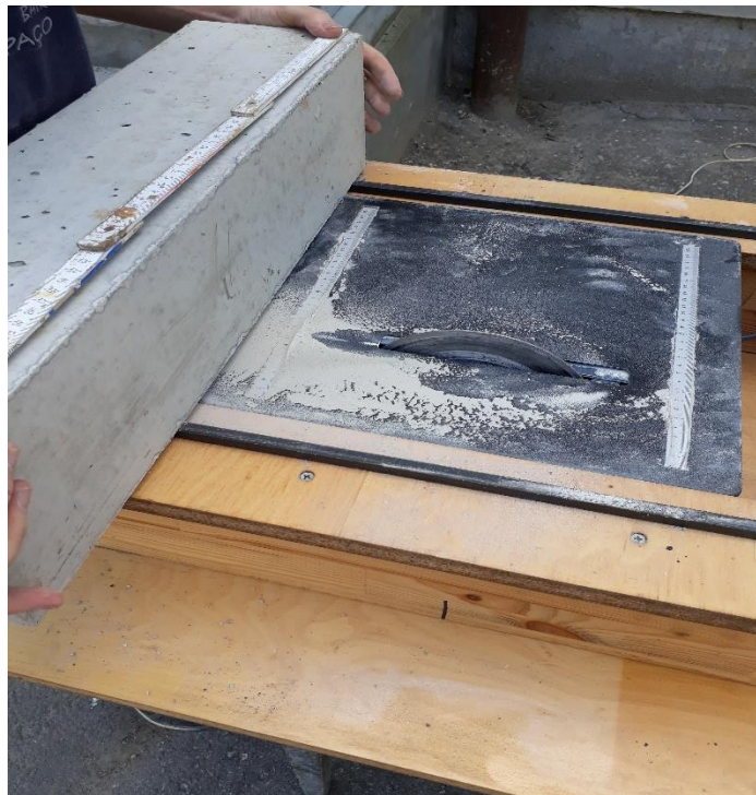
Figure 20: Cutting the fissure for specimen.
