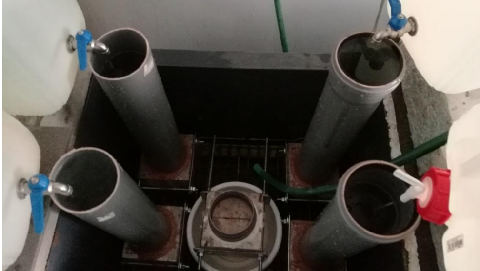
Figure 13: Testing procedure of crack healing effect
