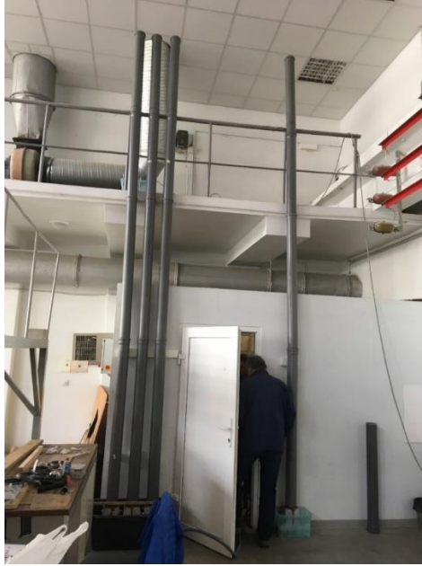
Figure 14: Testing procedure of crack healing effect with 5-meter high water column pressure (is about 0.5 atmospheric pressure on specimen).
