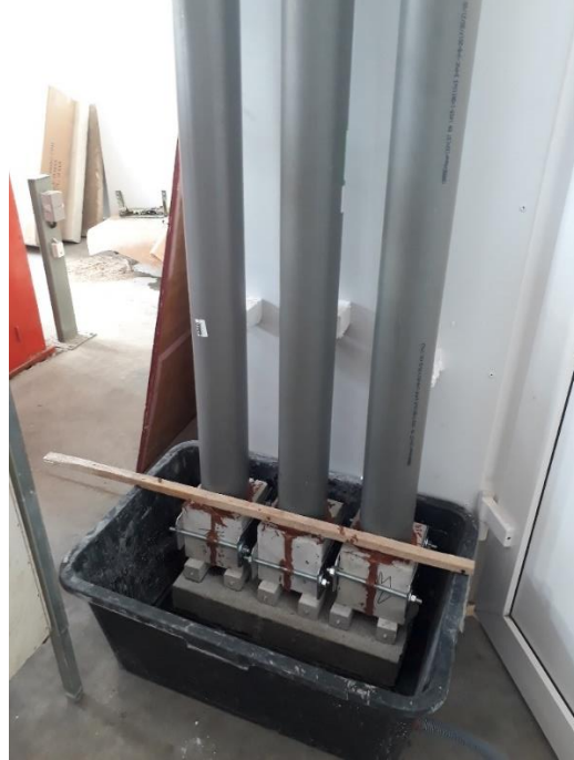
Figure 15 : Specimen fixed to 5m tubes.
