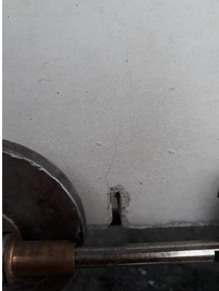
Figure 23: Crack start to shows.
