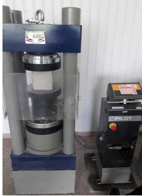
Figure 16: Crushing the cubes before putting in water.
