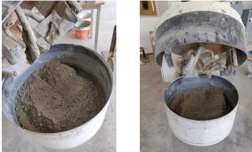
Figure 22 & 23. SCFRC concrete mixture
