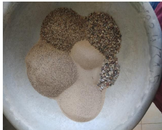
Figure 4 and 5. sieve analyzed of 1 mm and 4 mm fine aggregate
