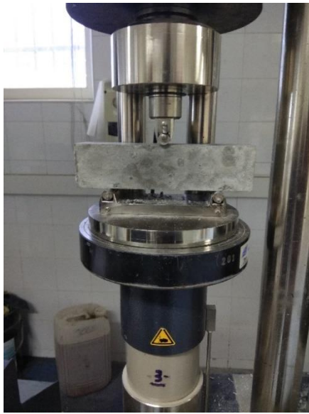
Figure 19&20. Flexural strength of SCC concrete replacement with PFA
