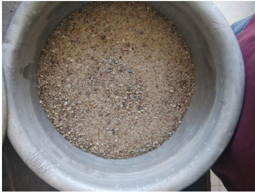
Figure 2 and 3. size of 0-4 mm and 0-1 mm fine aggregate
