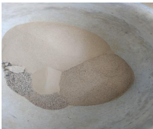
Figure 4 and 5. sieve analyzed of 1 mm and 4 mm fine aggregate
