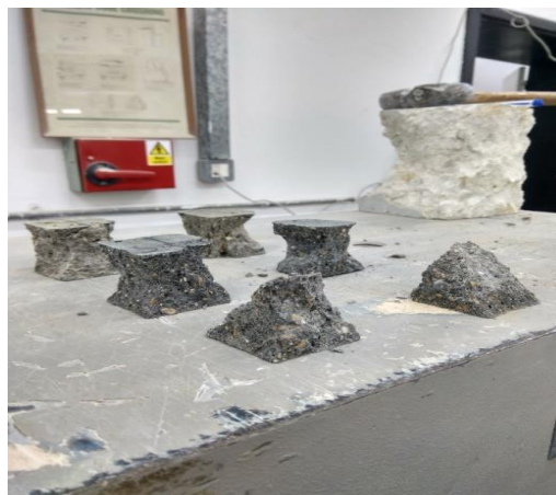
Figure 9, 10, 11. Crack deformation of prism after 3, 7, 28 days
