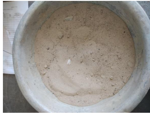
Figure 2 and 3. size of 0-4 mm and 0-1 mm fine aggregate
