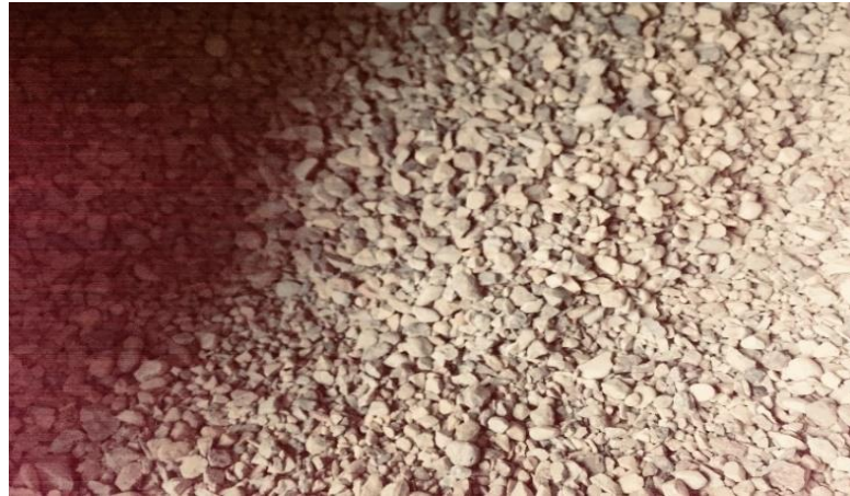
Figure 5: Course aggregate using in concrete mixing
