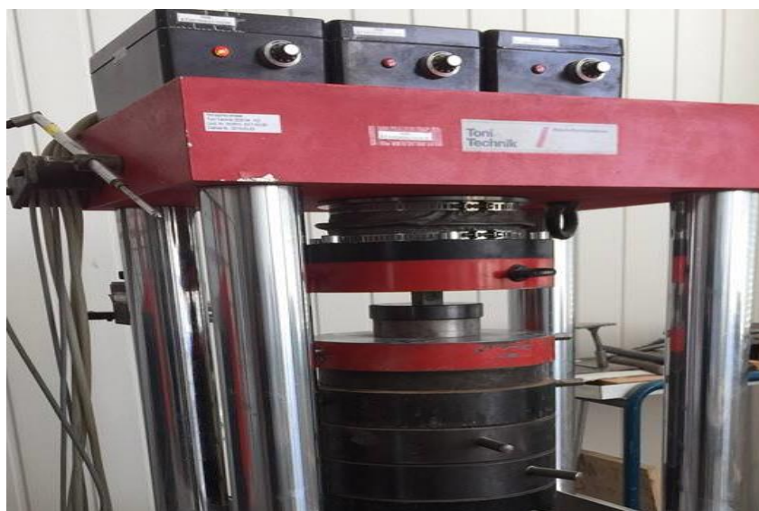
Figure 2: Compressive strength test of the hardened cement paste specimens
