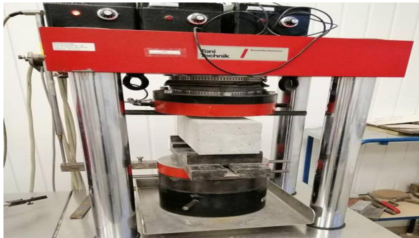
Figure 1: flexural concrete specimens test
