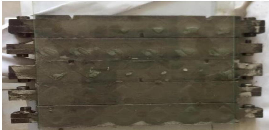
Figure 11: hardened cement paste specimens in the moulds
