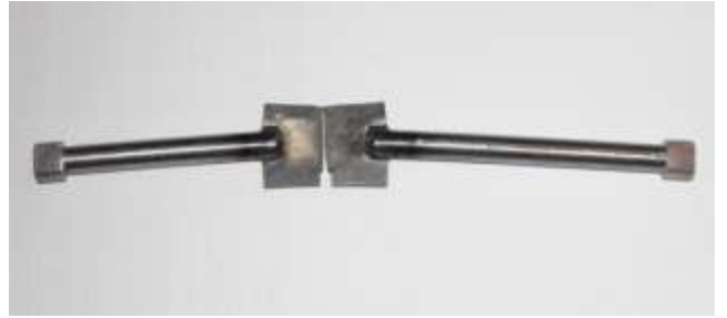
Fig. 3 Specimen with oblique angles slits every 5^\circ , starting from 0^\circ to 45^\circ
