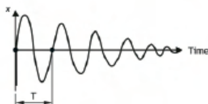
(c) The displacement of mid-span after someone jumps once at mid-span
