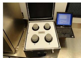
Fig. 1.4 Grace radical portable field calorimeters.[6]
