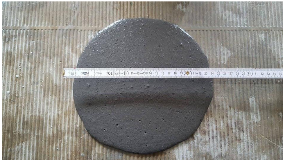
Fig. 3.3 Flowability of fresh concrete( W/c = 0.3 )
