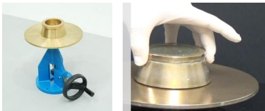
Fig. 1.9. Brass flow table test. [47]
