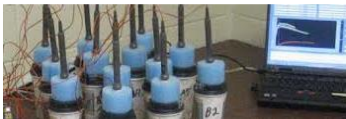
Fig. 1.3 Solidus Integration thermal system for “coffee cup” calorimetry.[6]
