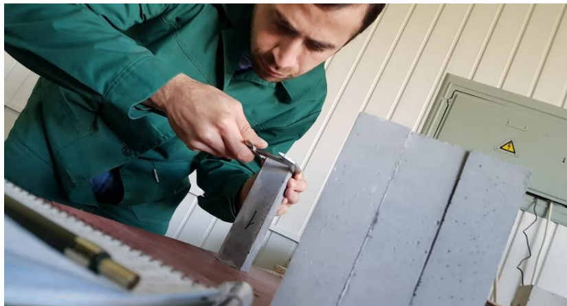
Fig. 3.4 Calculate the concrete density of samples.
