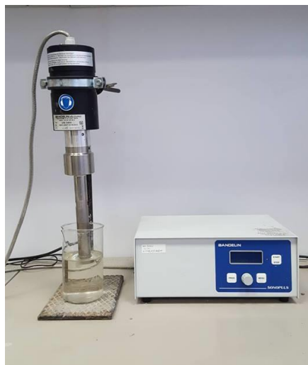
Fig. 3.2 Bandelin Electronic Ultrasonic Homogenizer UW 3400.
