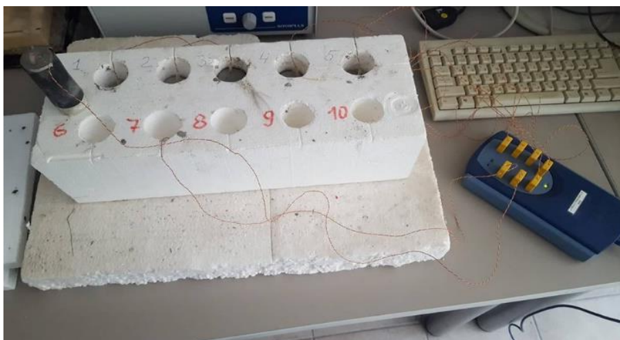
Fig. 3.1 Semi-Adiabatic Calorimetry test sample preparation.
