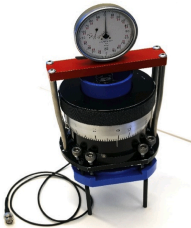
Fig. 13. Experimental chamber for assessment of water gap impact on the magnitude of reflected signal.
