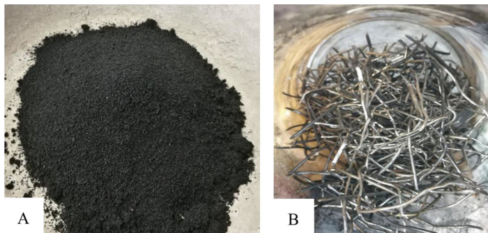
Fig. 3. Materials used in the study: (A) shredded tire-waste rubber obtained from recycled tires; (B) recycled tire steel cords.
