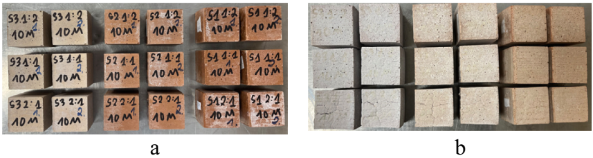
Fig. 1. Comparison of geopolymer mortar prior to heating (a) and after thermal exposure at 900 °C (b).
