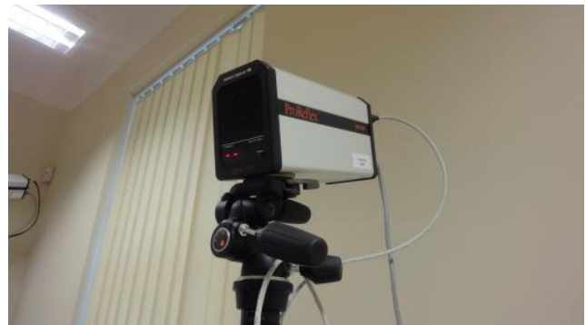
Fig. 1 ProReflex MCU 500 Type 170 214 camera
