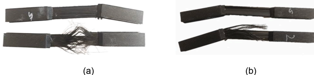
Fig. 6. Printed samples after tensile testing, (a) Tow A, (b) Tow B.
