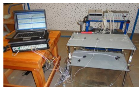
Fig. 1 Laboratory model of flooring building and experimental setup
