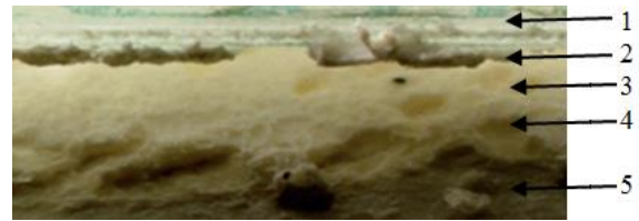
Fig. 3 Cross-section view of a passport's page fragment after forgery attempts using a mechanical method. 1 – Protective polycarbonate transparent layer; 2 – polycarbonate transparent layer for data recording after the change of primary content; 3, 4 – polycarbonate white layer after repeated gluing; 5 – Protective teslin layer after repeated gluing and/or fusion [Document Analysis Department at the State Border Guard Service]
