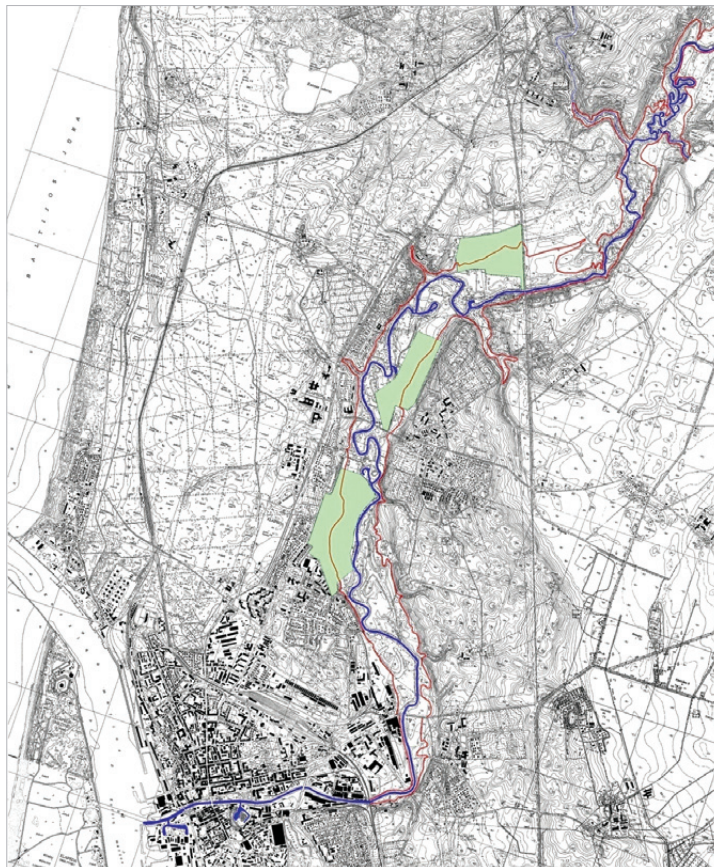
Fig. 6. Modeled flooded territories by the Akmena-Danė river within the City of Klaipėda and its suburbs (10–12 August, 2005) under the combined impact of stormy runoff and marine water surge. Red line shows maximum flood extent but flooded residential and recreational areas are shadowed by green
