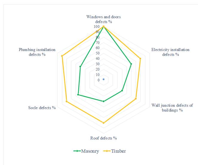
Figure 4. Defects of houses indicated during inspection
