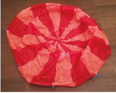
FIGURE 10: The 16-segment, dome-shaped parachute.
