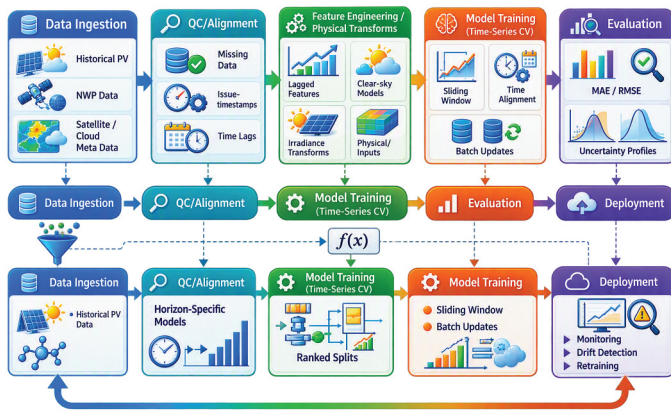
Figure 5. Generic PV power forecasting workflow shared across physical, statistical, and learning-based approaches.
