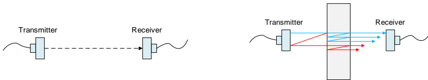
Fig. 2.25. Measurement setup: without sample (left) and with sample (right)
