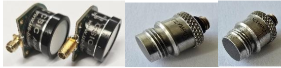
Fig. 92. Transducers used in investigation: (left) air-coupled and (right) immersion
