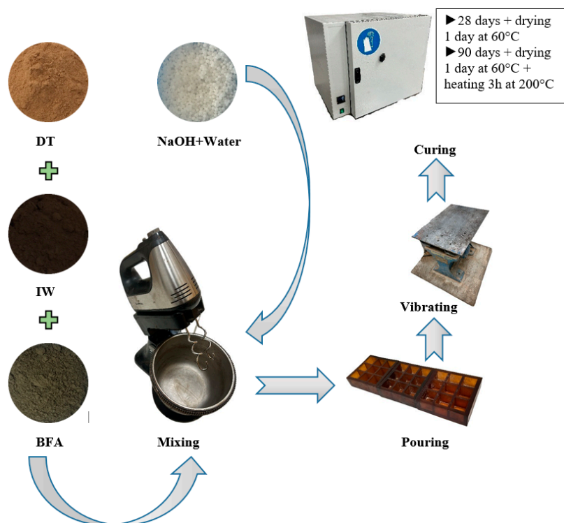
Figure 6. Order of the sample preparation steps. The arrow \Rightarrow indicates the order in the preparation of the samples. The arrow \blacktriangleright refers to the curing conditions for the test samples.
