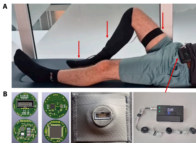
Fig. 8. The limb activity module for tracking lower-limb kinematics using inertial measurements. (A) A prototype wearable integrating 3 activity sensors positioned on the right thigh, shin, and foot. (B) From left to right: single sensor printed circuit board rendering (20 mm in diameter); indicative sensor integration within the wearable; and integrated sensors and controller for powering and controlling up to 7 sensors.
