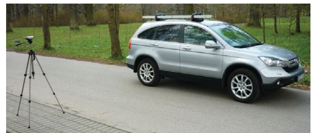
Fig. 3. System for precise velocity measurement with laser
