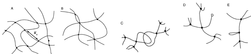
Fig. 2. Different types of network bond. A) Ideal macromolecular network, B) real networks with multifunctional bonds, C) physical molecular entanglements, D) unreacted functionalities with partial entanglements, E) chain loops [35]
