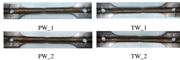
Fig. 4 Photos of the flat welded specimens (series PW) and the welded tube contoured specimens (series TW) after fracture
